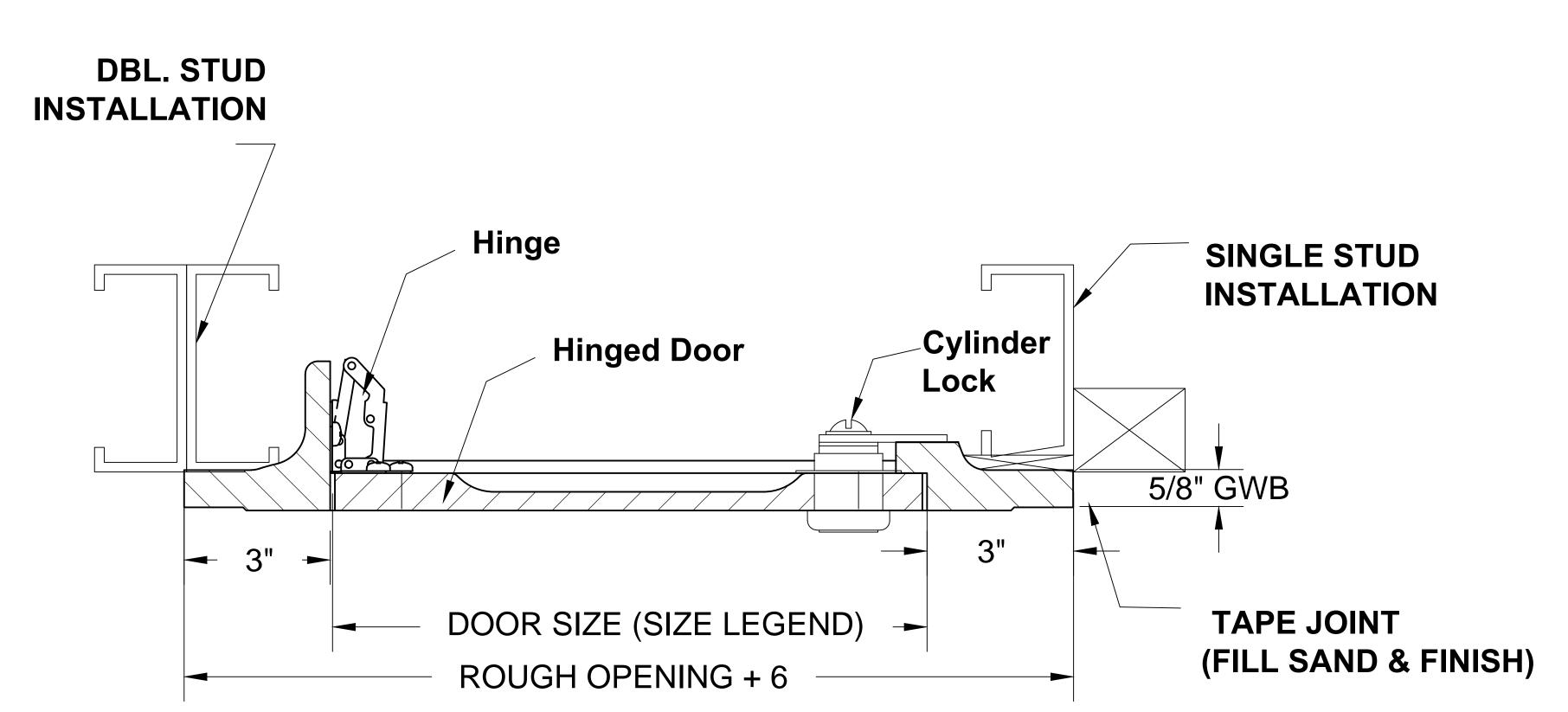
Access Panel - Side View (Single/Double stud installation)
