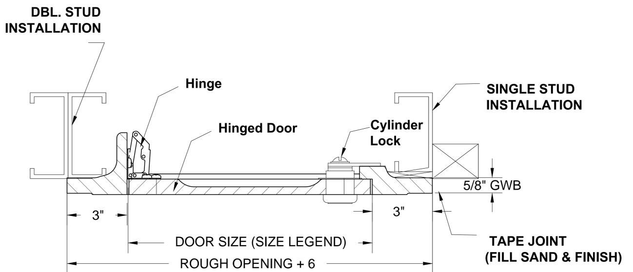
Access Panel - Side View (Single/Double stud installation)
