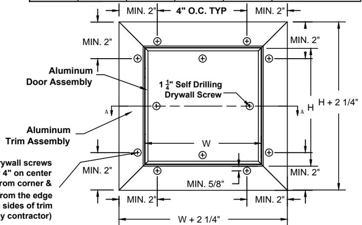
Use 1 1/4" self drilling drywall screws approximately 4" on center and MIN. 2" from corner & MIN. 3/8" from the edge on all 4 sides of trim (supplied + installed by contractor)
